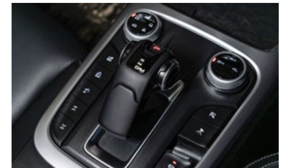
ALL-TERRAIN PROGRESS CONTROL (ATPC) SYSTEM
